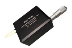
Agiltron's Manual Grating-Based Fiber Optic Tunable Filter provides a simple way to adjust the center wavelength of a narrow band over a wide band. Wavelength tuning is achieved by rotating a grating using a micrometer.
